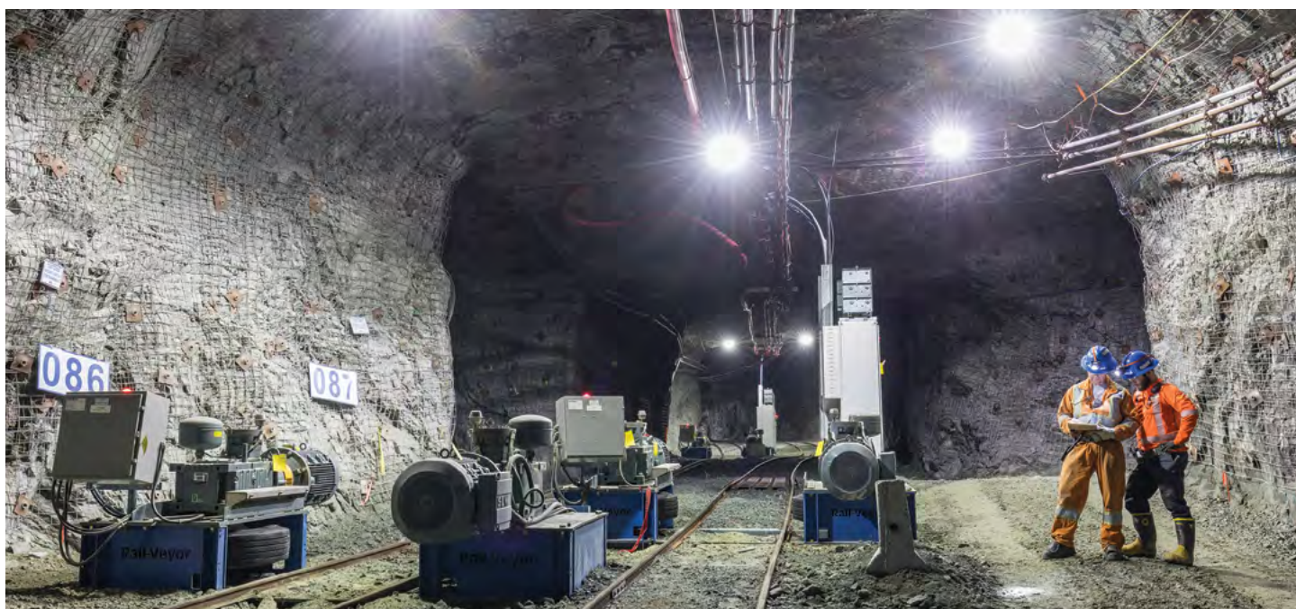
The new Rail-Veyor ore transportation system at Agnico Eagle's Goldex Mine in Quebec.
