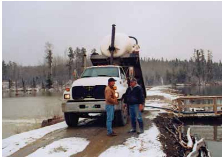
Adding lime to neutralize Thompson tailings water
