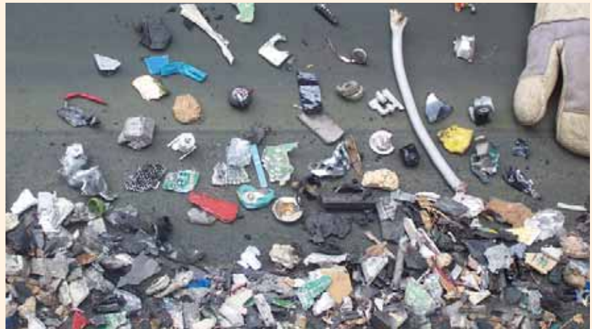
E-waste close-up on feed belt
